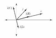
b)  $i_R = \frac{v}{\pi}$  is always in phase with the voltage.  $i_L = \frac{v}{\omega L}$  lags the voltage by 90°, and  $i_C = v\omega C$  leads the voltage by 90°.
